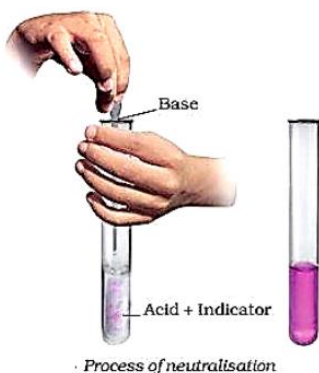
Figure 9: Neutralization using Phenolphthalein
