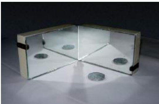
Fig.10 : Images in plane mirror at right angle to each other
